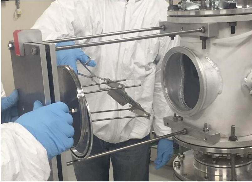
1 2 Figure 5. Insertion of the ^7\text{Be} radioactive target in the setup, with a support independent of the telescope detector 3 installed from the opposite side of the chamber.
