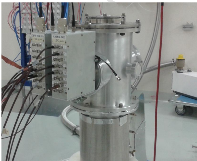
Figure 3. The scattering chamber, with the front-end electronics, installed on the vertical neutron beam line in EAR2. The target and the telescope detector are inside.
