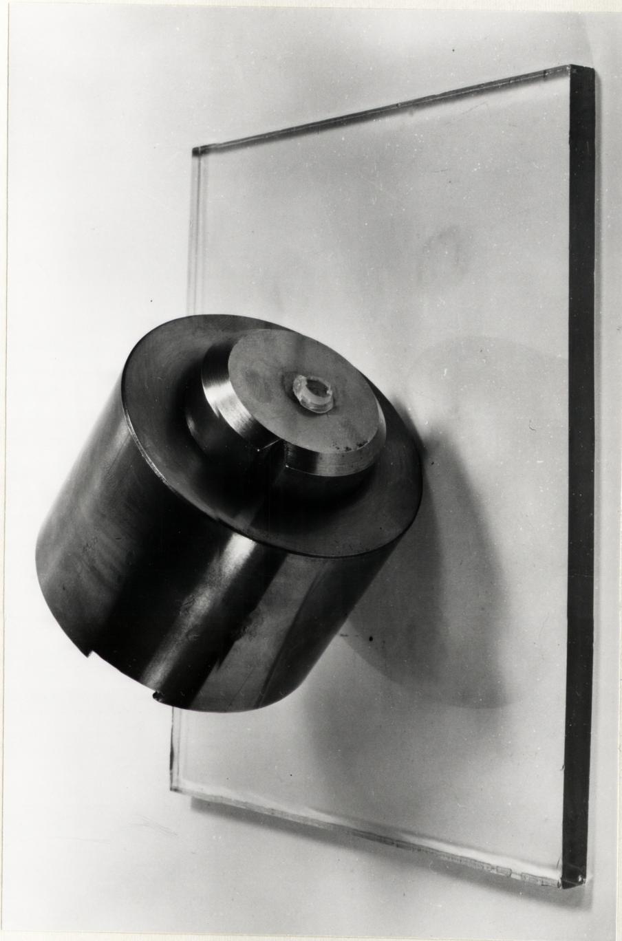
Fig 3.10 Precision grinder used in ^{133}\text{Ba} diffusion study
