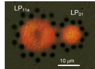
Figure 2. Cross-section of PMMA holey fibre mode-selective coupler showing mode coupling when using a broadband source.
