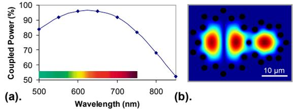
Figure 1. (a) BPM calculated [5] wavelength dependent power transfer between the LP<sub>01</sub> mode of the smaller core and the LP<sub>11a</sub> mode of the larger core of the holey fibre mode-selective coupler shown in (b).
