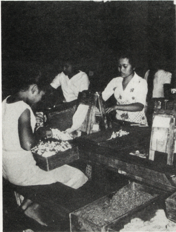
Plate 6.7 Kretek rolling machine, 3000-7000 kretek per operator per day.
