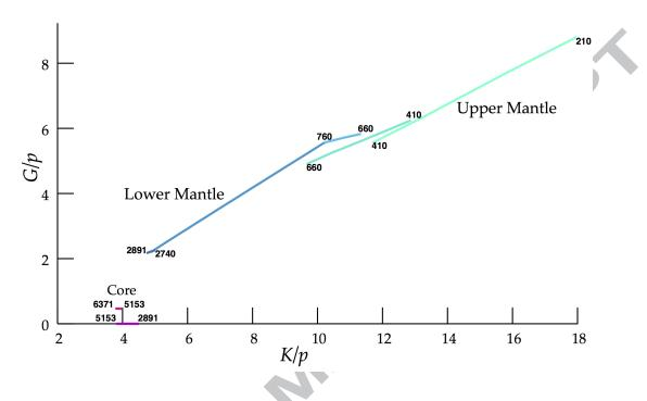
Figure 1: Multiple linear segments for the relation between G/p and K/p for different parts of the *ak135* Earth model (Kennett et al., 1995). The depths for each segment are indicated. Multiple depths indicate the presence of major discontinuities.
