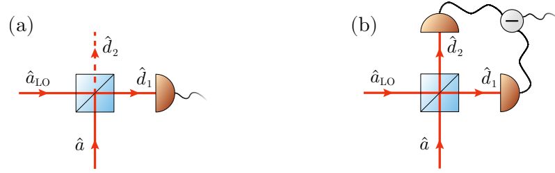
Figure 2.7: Schematic of a homodyne/heterodyne detection setup. (a) Combination and detection of the signal field with a reference local oscillator. (b) A clean quadrature measurement is obtained after subtracting the read-outs of photodetectors at both ports.
