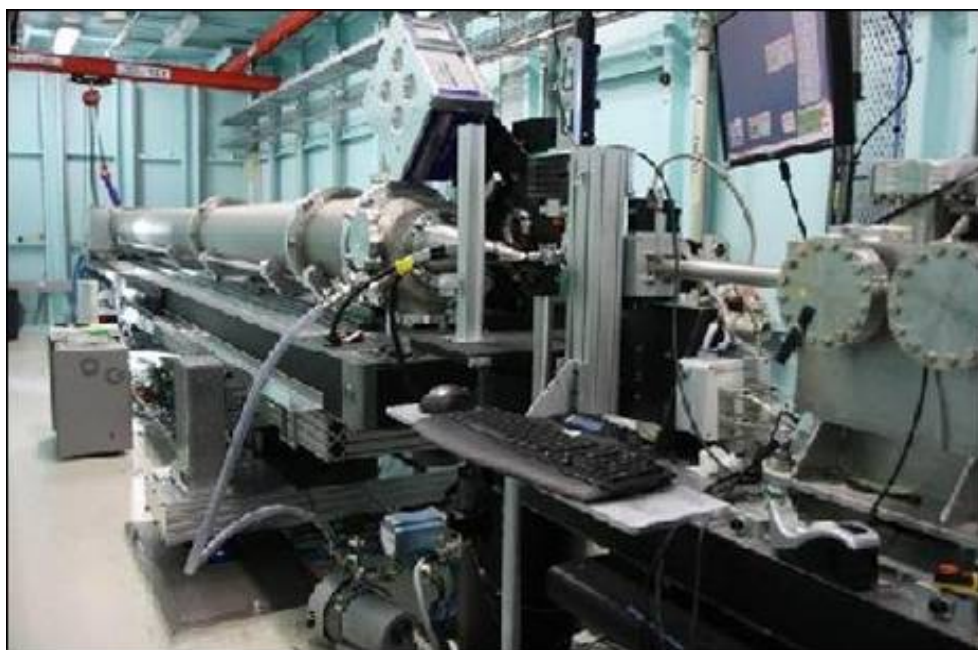
Figure 3.12: Photo of the SAXS/WAXS beamline of the Australian Synchrotron. (Image courtesy: Australian Synchrotron)
