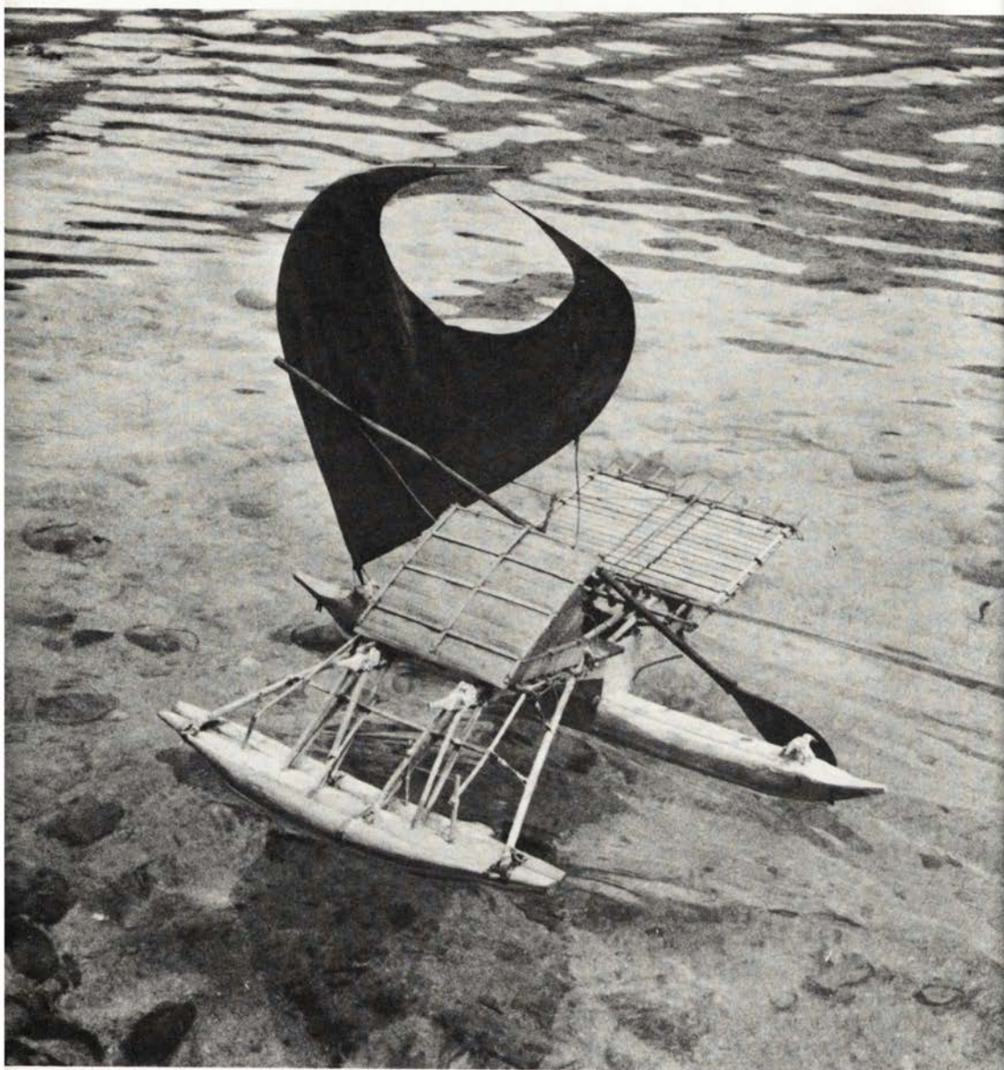
Plate II Scale model of 40-foot te puke as used by Tevake. Photographed at Taumako.
