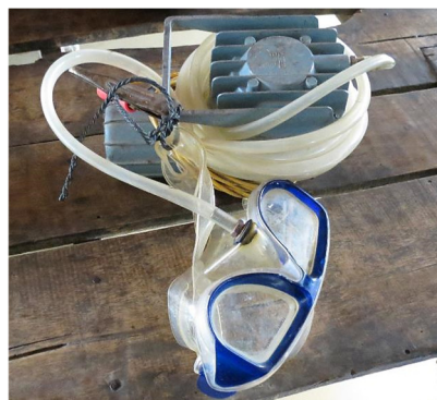
Figure 5.5 A diving device created by a prawn farmer in Phu Thanh B
