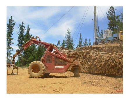
Figure 3.5 Use of "three-wheels" (ergo logger) in medium-sized forest operations. Source: courtesy of the Forestry and Timber Forum.
