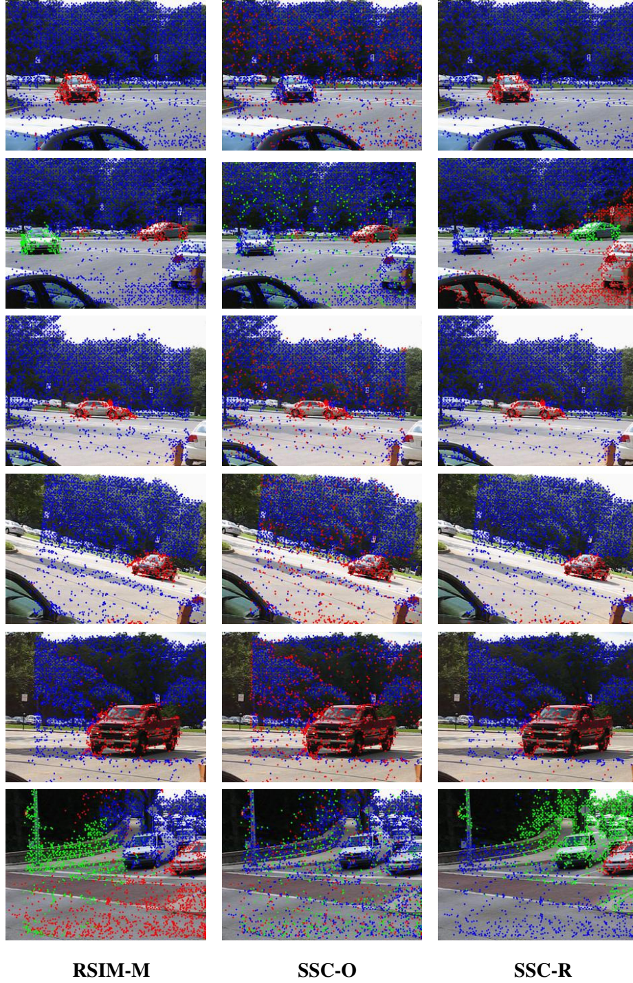
Figure 4.9: Semi-dense motion segmentation results for sequences 5-10. Our method (RSIM-M) uses all the available tracks ( 3026 on average ) with an average runtime of 5.22 seconds per sequence ; SSC-O tends to group the trajectories with missing entries in the same cluster; SSC-R takes 150.48 seconds on average and only makes use of 2522 points on average after removing the incomplete trajectories. Best viewed in color.
