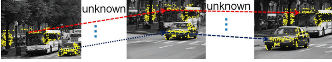
Figure 5.1: Motion segmentation with unknown correspondences: given a video sequence and feature points in each frame, our goal is to simultaneously estimate motion clusters and feature matching.
