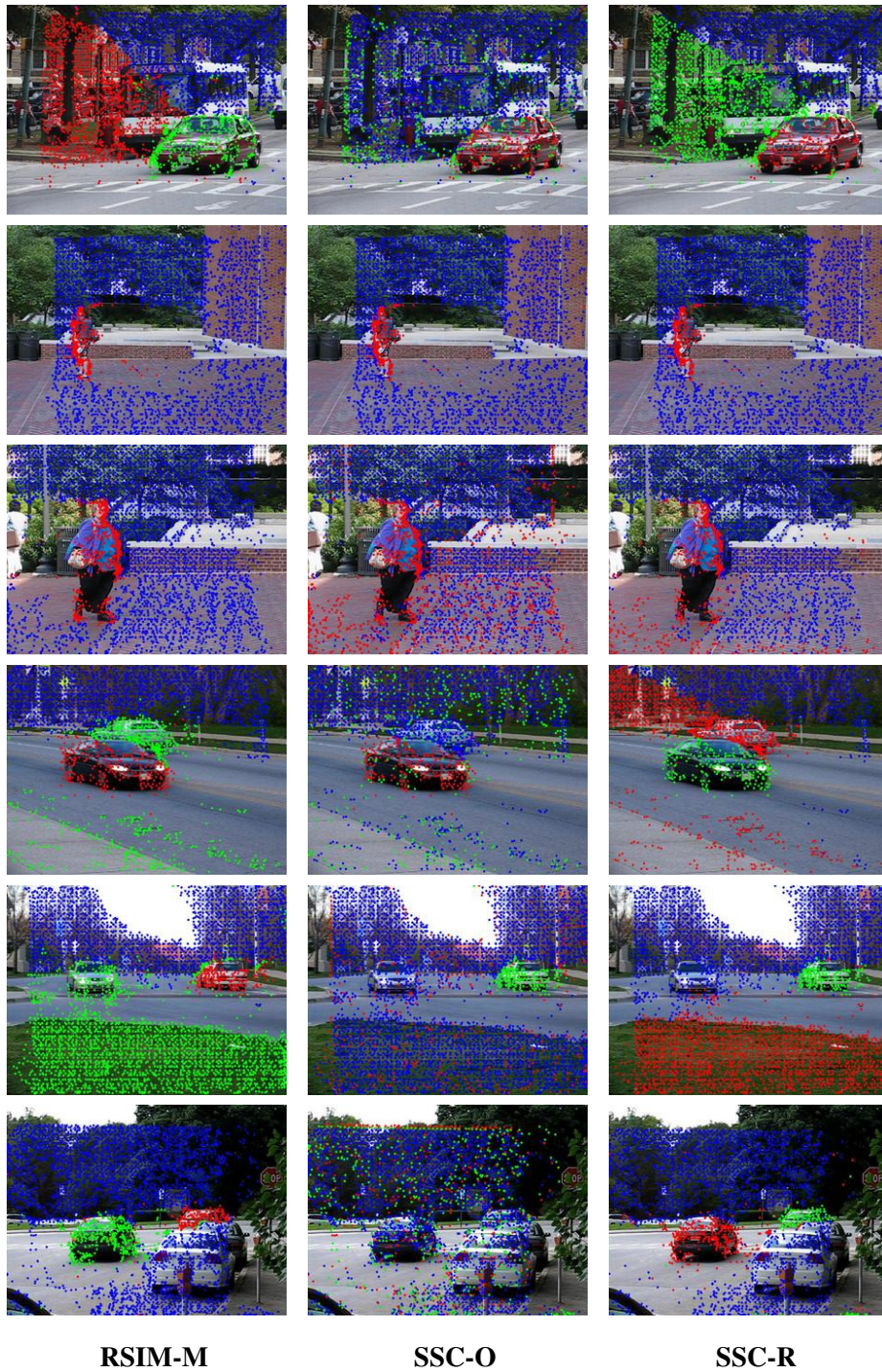
Figure 4.10: Semi-dense motion segmentation results for sequences 11-16. Our method (RSIM-M) uses all the available tracks ( 3026 on average ) with an average runtime of 5.22 seconds per sequence ; SSC-O tends to group the trajectories with missing entries in the same cluster; SSC-R takes 150.48 seconds on average and only makes use of 2522 points on average after removing the incomplete trajectories. Best viewed in color.
