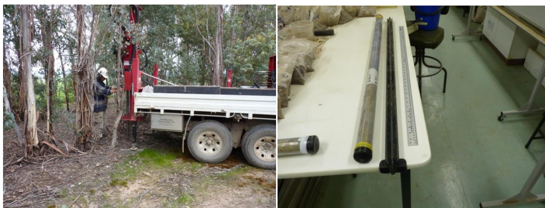
Figure 3-1. Where access was possible within BEPs, soil cores were collected using a truck mounted Dingo Ezi Probe mechanical corer by a PVC sheath.
