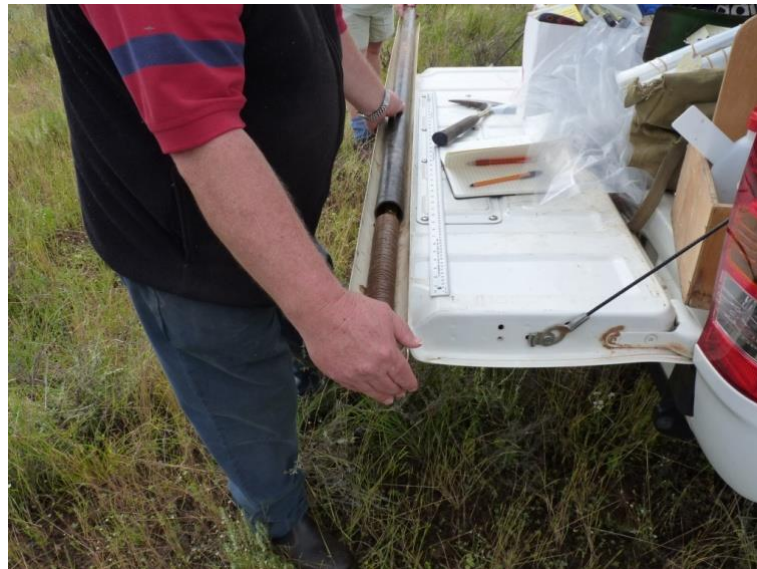
Figure 3-3. The soil sample was gently pushed out of the steel sheath to allow slicing the sample into depth increments
