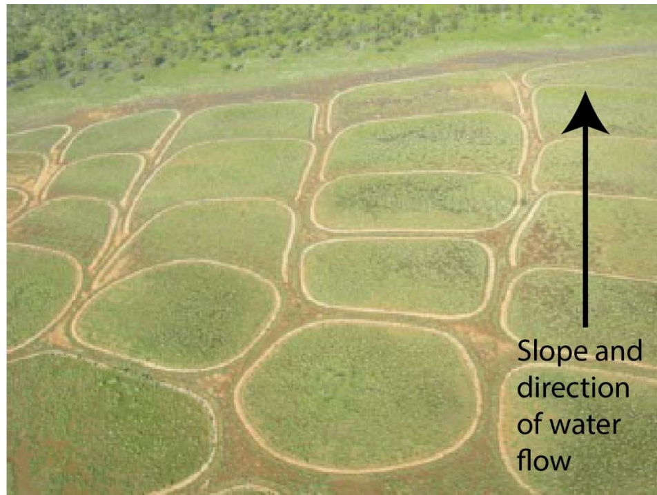
Figure 5-5. Aerial photograph showing a network of horseshoe shaped and fully enclosed waterponds. Fully enclosed waterponds are established where the surface is flat, horseshoe shaped waterponds are established on sloping surface. (Source: R. Thompson).
