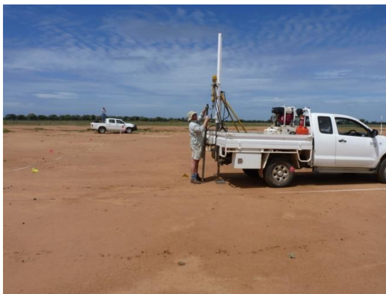
Figure 5-11. Soil coring rig used for sample collection on scalds and waterponds.
