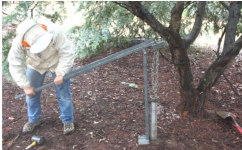
Figure 3-2. Method used to manually extract a soil core within BEPs (photo: C. Vuillot).
