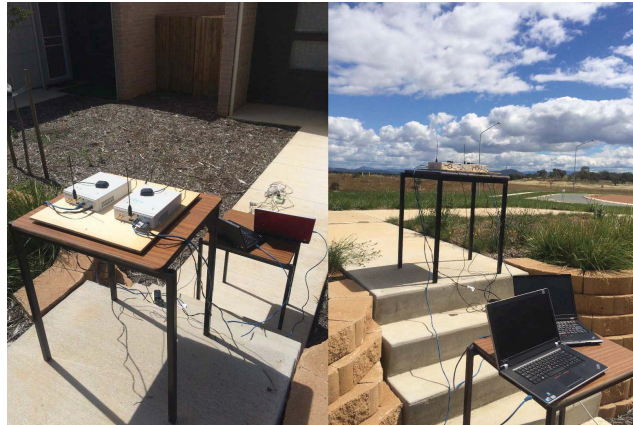
Figure 4.5: Experimental setup of two co-located SDRs
