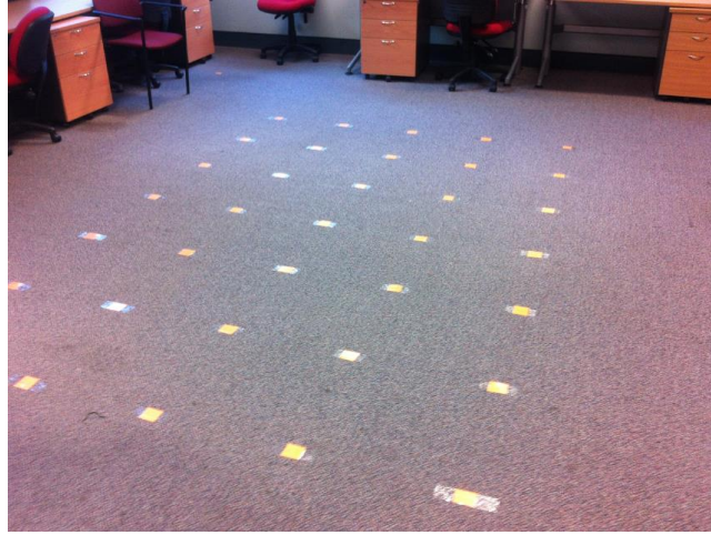
Figure 3.12: Marks on the intersection of grid lines in indoor area
