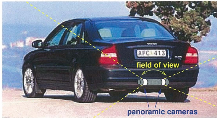
Figure 3.10: A conceptual drawing showing how the final panoramic sensor could be mounted to a production car.
