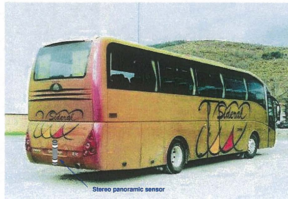
Figure 3.12: The stereo panoramic sensor mounted at the rear of a bus.
