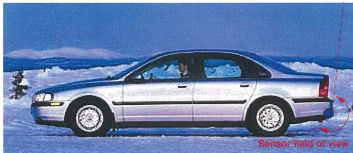
Figure 3.10: A conceptual drawing showing how the final panoramic sensor could be mounted to a production car.
