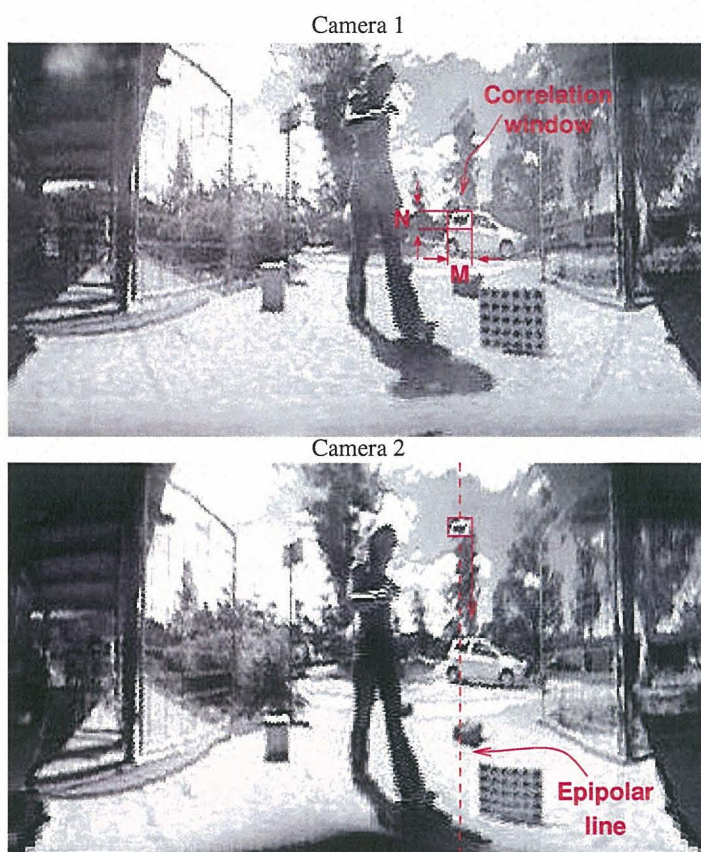
Figure 4.3: Computing disparity using an area based method.
