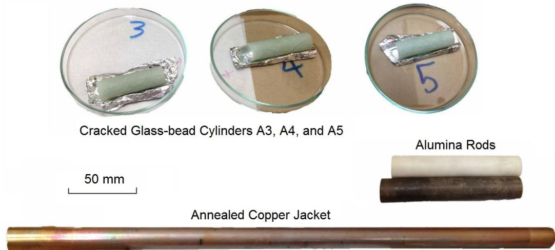
Figure 3.8 Cracked low-porosity (~2%) glass-bead cylinders (labelled as A3, A4, and A5) and two alumina rods, all of which need to be inserted into an annealed copper jacket to form a specimen assembly.
