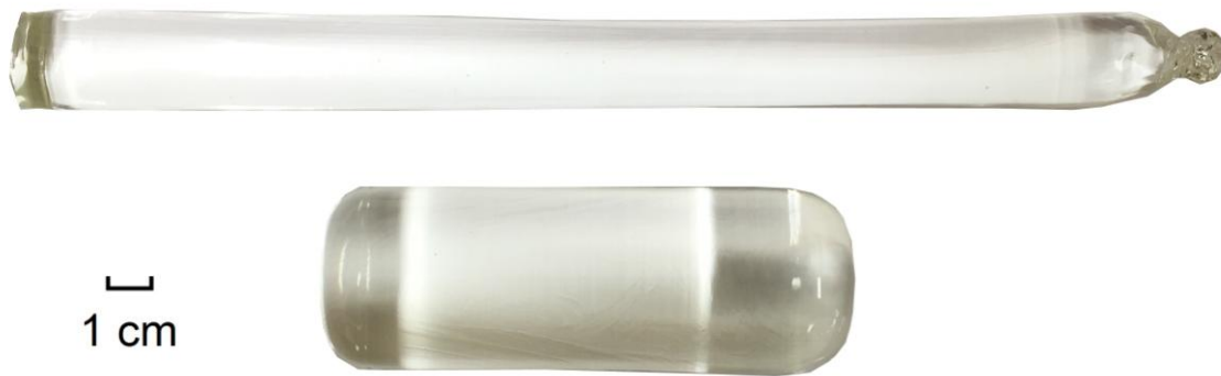
Figure 2.2 The raw soda-lime-silica glass rods with a diameter of either ~ 20 mm (upper) or ~ 40 mm (lower), which were later precision ground into cylindrical specimens for measurements.
