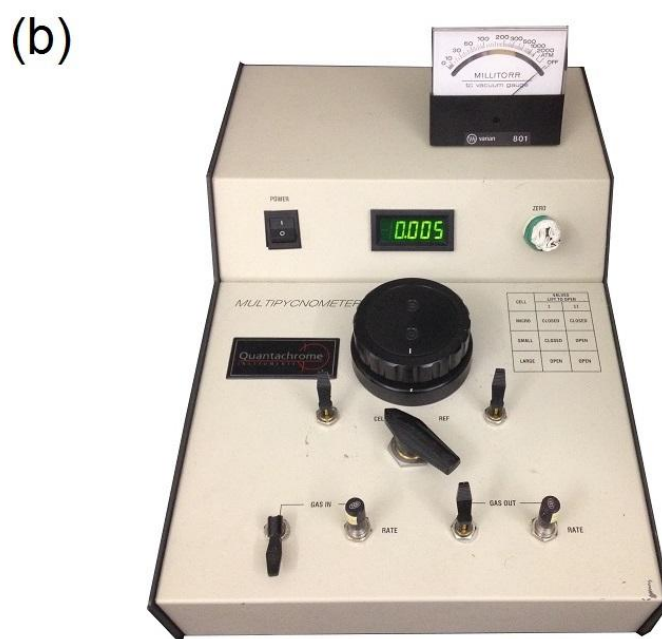
Figure 2.12 a) The arrangements of the MVP-D160-E type helium pycnometer. b) A photograph of the helium pycnometer in the Rock Physics Laboratory at the University of Alberta.
