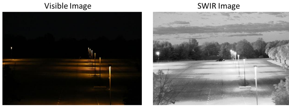
Figure 1.5 The same photo taken during the night using (a) a normal camera (b) using a SWIR camera. http://www.sensorsinc.com/gallery/images .
