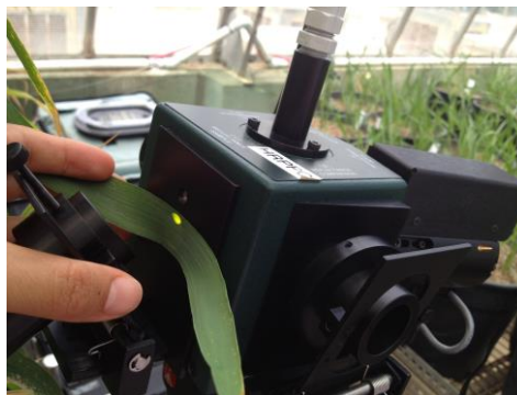
Figure 4.4 Measuring reflectance with the ASD fieldspec 3 coupled to the integrating sphere in a flag leaf of wheat.
