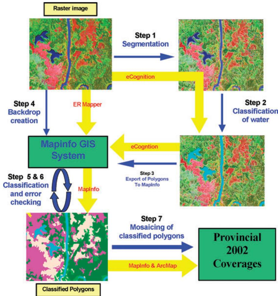
FIGURE 2. The process of image classification showing the seven principle steps.
