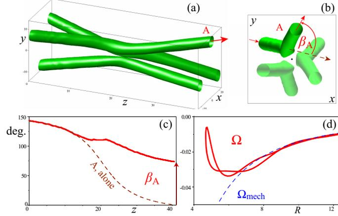
Fig. 3. Calculated dynamics of three beams in saturable media (Media 4). (a) 3D and (b) transverse views of the interacting beams showing their twist due to interaction. The twist is characterized by the angle  $\beta_A$  (c) and by the angular velocity  $\Omega$  (d).
