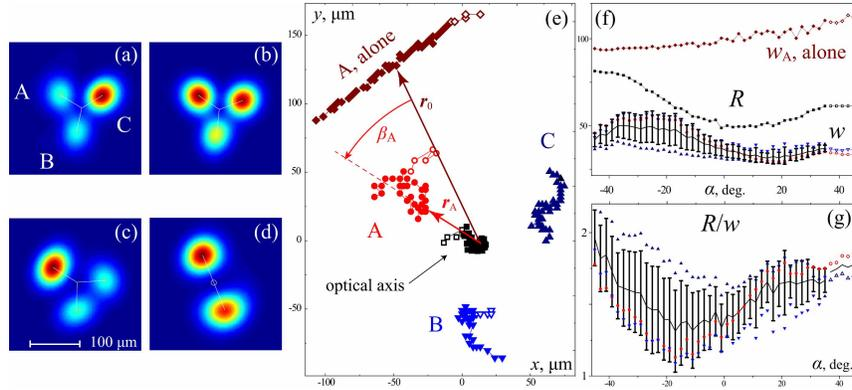
Fig. 4. Three lobe azimuthon experiments. (a-d) Measured output profiles for input tilts  $\alpha = 1^\circ, 15^\circ, 29^\circ, 43^\circ$  and power  $690 \mu\text{W}$ . (e) Output positions of the three lobes compared with the position of a single noninteracting lobe, marked “A, alone”. The azimuthon radius  $R$  and the average width of each beam  $w$  are shown in (f) and their ratio in (g).
