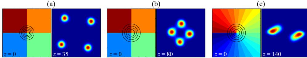
Fig. 1. Numerical results on phase imprinting: (a, [Media 1](#)) four-lobe unstable soliton cluster; (b, [Media 2](#)) four-lobe localised azimuthon formation; and (c, [Media 3](#)) unstable vortex soliton. Left: input phase profiles with superimposed intensity contours of the Gaussian beam. Right: intensity profiles after propagation distance indicated in the images.
