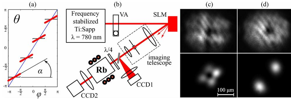
Fig. 2. (a) Phase distribution for generation of azimuthons. (b) Experimental setup: VA - variable attenuator, SLM - spatial light modulator, Rb - Rubidium cell,  $\lambda/4$  - quarter waveplate, CCD - cameras. (c, d) Experimental results: Input (top) and output (bottom) intensities for (c) an azimuthon with  $\alpha = 0^\circ$  and (d) vortex with  $\alpha = 45^\circ$ . Input power  $830 \mu\text{W}$ .
